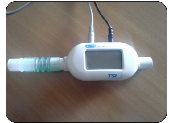
Flow meter in continuous mode to analyze the air flow from ventilator to patient
